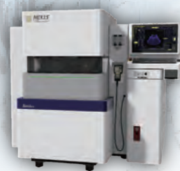
MEX15 Oil-spec ultra-precision machine applicable for \Phi 0.03 wire
